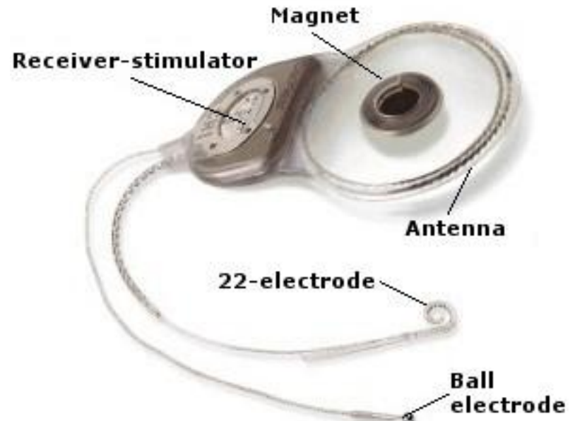
Figure 1. The internal component of the cochlear implant
